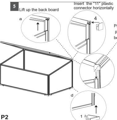
Press the plastic connector into side board vertically
