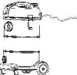
To use the flexible hose, insert the end of the hose into the suction hole. Make sure, that it is snapped in the position.
