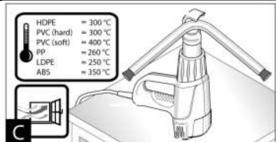
**Plastics welding** Install the reduction nozzle (11) and the welding foot on the gun. The workpieces to be welded and the welding wire must be of the same material. The weld must be clean and free of grease. Carefully heat both welds until they reach a melted consistency. When working, be careful and remember that the thermal difference between the molten and liquid consistency of the plastic is small. Add the welding wire and let it melt
